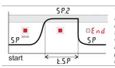
*Timer mode 6:* In this mode, the temperature is maintained at the set-point temperature SP.2 as long as the timer is running. The timer is started when the process temperature is within the adjusted tolerance band. When the timed period has elapsed, the KS 40-1 returns to the initial set-point.
